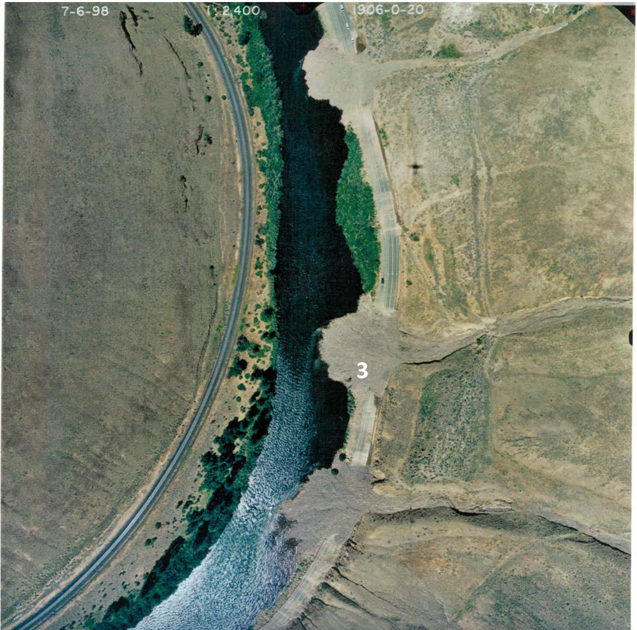
Figure 21. Vertical aerial photograph of the Stop 3 site. Note the large debris fans extending into the Yakima River. Bold number indicates field trip stop site. Source: Washington Department of Transportation, 6 July 1998.
