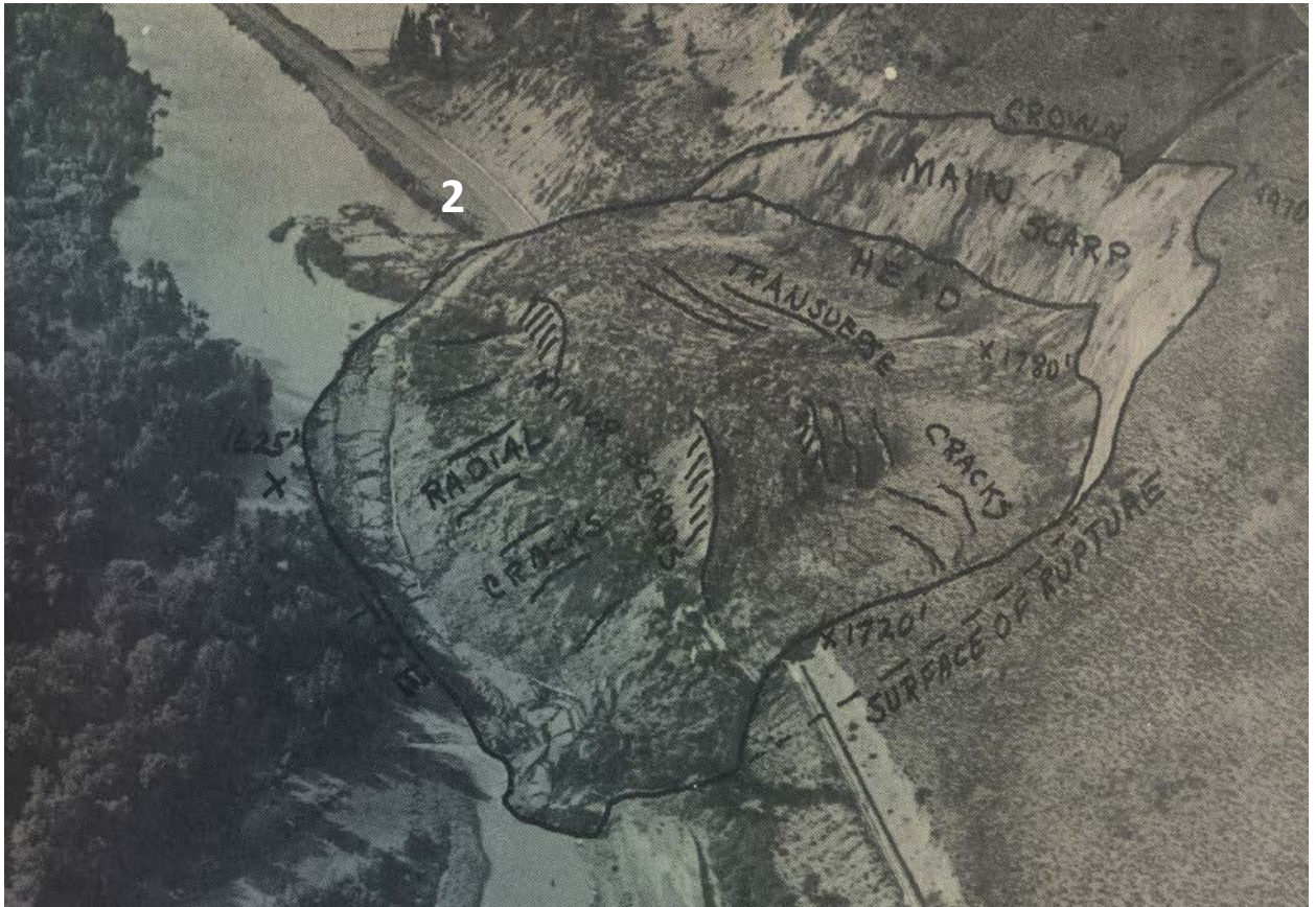
Figure 14. Annotated oblique view upriver (west) at the June 1970 landslide near Milepost 101, WA 10. Cars are parked at bold 2. Source: Kaatz (1971).
