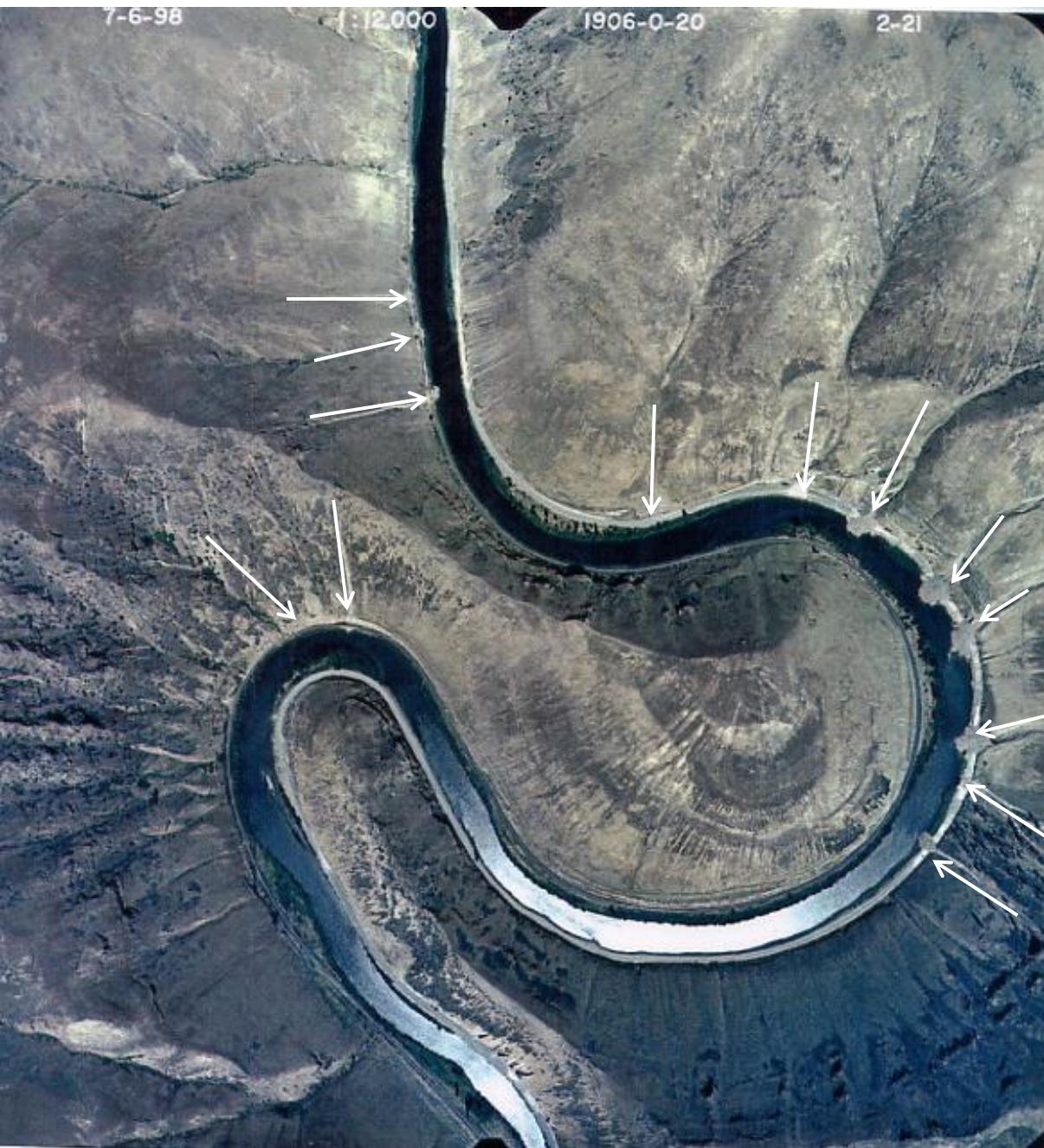
Figure 13. Debris fans of 3 July 1998 debris flows, Yakima River Canyon. Arrows indicate debris flows that reached State Route 821 or Burlington Northern Santa Fe railroad. Washington Dept. of Transportation photo.
