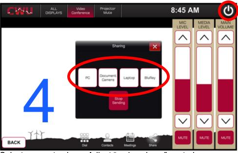
Select source to share. Adjust "main volume" control. Power off the system when class has finished.
